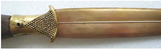
Figure 14. Dagger #30-12-550, PG 1054 from the Royal Cemetery of Ur, 2500–2000 BCE. The dagger has been depletion gilded and is made of a gold, copper, and silver alloy. Metallurgic analysis was performed in 2009 at the Penn Museum (Zettler et al., 2017).
